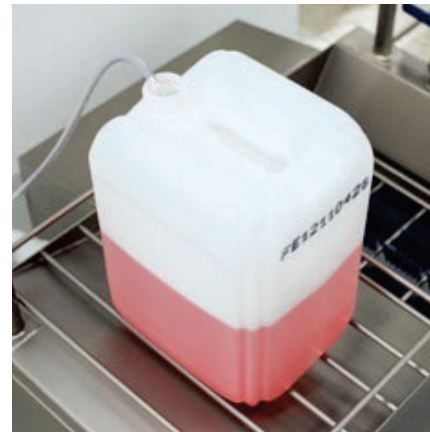
Storage grating for cleaning detergents
